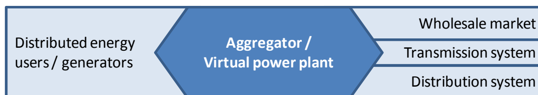
Figure 7. Schematic view of a virtual power plant
